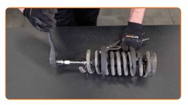
18 Remove the rubber spring spacer.
