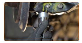
Tighten the fastener connecting the control arm to the rear subframe. Use a combination spanner #19. Use a drive socket #19. Use a torque wrench. Tighten it to 90 nm torque.
