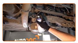
Loosen the fastener connecting the control arm to the rear subframe. Use a combination spanner #19. Use a drive socket #19. Use a tap wrench.
