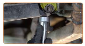
Install the coil spring compressor on the coil spring.
