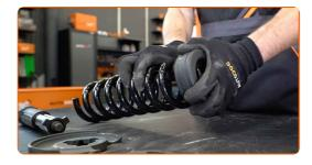
Install a new coil spring on the coil spring compressor.
