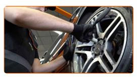
Lower the car and working in a cross order, tighten the wheel bolts. Use wheel impact socket #17. Use a torque wrench. Tighten it to 112 Nm torque.
