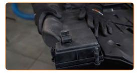
Screw in the fasteners of the air filter covers. Use Torx T20. Use a ratchet wrench.
