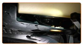
Slide the cabin filter retainer to release it.
