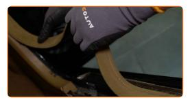
Λ Remove the side panel on the passenger side.
