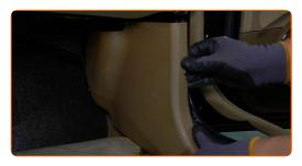
Unscrew the fasteners of the passenger side kick panel. Use Torx T20.
