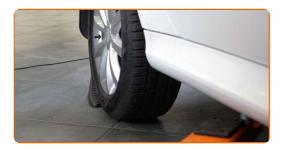
Loosen the wheel mounting bolts. Use wheel impact socket #H12.
