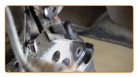
Install a new rod, tighten the fasteners. Use a combination spanner #16. Use a drive socket #16. Use a drive socket #8.
