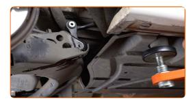
Tighten the fastener connecting the stabilizer bar with the control arm. Use a combination spanner #16. Use a drive socket #16. Use a torque wrench. Tighten it to 40 Nm torque.
