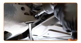
Unscrew the fasteners connecting the stabiliser link to the stabiliser bar. Use a combination spanner #16. Use a drive socket #8. Use a ratchet wrench.
