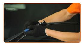
Remove the blade from the wiper arm.
