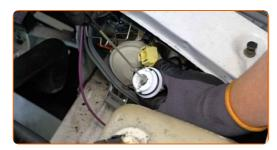
13 Install a new turn signal light bulb in the socket.
