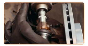
Tighten the tie rod end locknut. Use a combination spanner #19. Use a combination spanner #22. Use a torque 18 wrench. Tighten it to 50 nm torque.
