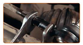
Connect the tie rod end to the steering knuckle. 16
