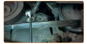
Place the V-ribbed belt on the tensioner pulley. Return the tensioner pulley to its initial position.
