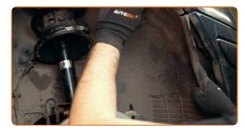
Install and tighten the wheel arch cover fasteners. Use a combination spanner #13.
