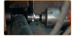
Treat the shock absorber mounting seats. Use copper grease.
