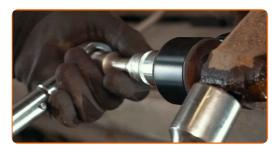
Remove the support from under the rear axle beam. 22
