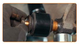
Screw in the lower fastener of the shock absorber. Use a drive socket #21. Use a ratchet wrench.
