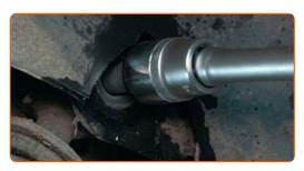
11 Remove the fastening bolt.
