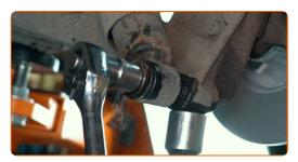
9 Remove the fastening bolt.
