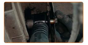
Screw the upper fastener of the shock absorber. Use 12-point socket No.21. Use a ratchet wrench.
