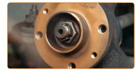
64 Install the brake disc.
