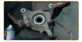
Press the hub out of the steering knuckle. Use a bush and bearing driver set.
