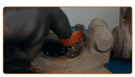
Remove the wheel hub bearing retaining ring. Use a flat screwdriver. 32
