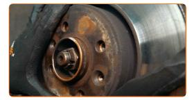
Tighten the brake disc fastening. Use Torx T40. Use a torque wrench. Tighten it to 14 Nm torque.
