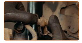
Treat all tie rod end connections. Treat the shock strut fasteners. Treat the fasteners of the ball joint. Use copper grease.
