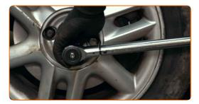
Tighten the wheel bolts using a criss-cross pattern. Use wheel impact socket #19. Use a torque wrench. Tighten it to 90 Nm torque.
