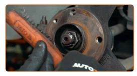
Treat the contacting surface. Use copper grease.
