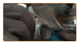
Press-fit a new bearing into the wheel hub. Use a bush and bearing driver set.
