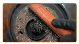
Unscrew the brake disc fastening. Use Torx T40. Use an impact screwdriver.
