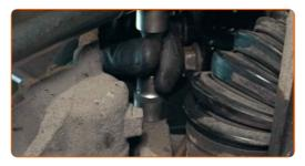
Connect the brake hose fastener to the suspension strut.
