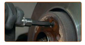
15 Remove the brake disc.
