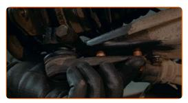
Screw in the fastener connecting the ball joint to the control arm. Use a combination spanner #18. Use a drive socket #18. Use a ratchet wrench.
