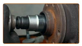
Detach the driveshaft from the steering knuckle. Remove the fastening bolt.
