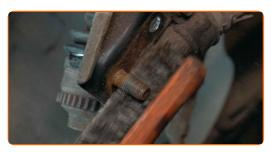
Treat the splines of the driveshaft CV joint. Treat the fasteners of the ball joint. Use copper grease.
