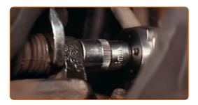
9 Remove the brake caliper.
