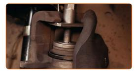
27 Install the brake caliper and fix it.
