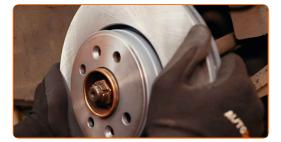
Tighten the brake disc fastening. Use Torx T40. Use a torque wrench. Tighten it to 14 Nm torque.
