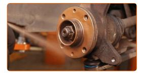
19 Install the brake disc.
