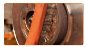
Unscrew the brake disc fastening. Use Torx T40. Use a ratchet wrench.
