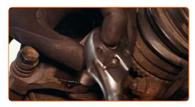
Remove the caliper bracket.
