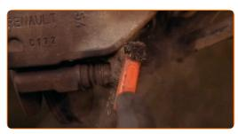
Unscrew the brake caliper fastening. Use a combination spanner #17. Use a drive socket #13. Use a ratchet wrench.
