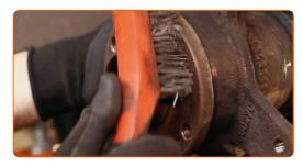
Treat the contacting surface. Use copper grease.
