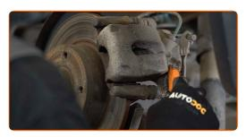
Unscrew the brake caliper fastening. Use a combination spanner #15. Use a drive socket #13. Use a ratchet wrench.
