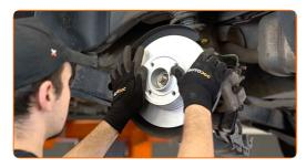
Screw the wheel hub lock nut. Use a drive socket #30. Use a torque wrench. Tighten it to 175 Nm torque.
