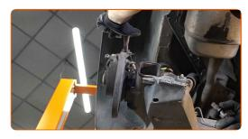
Pry up and remove the wheel hub cap. Use a crowbar. Use a hammer.
