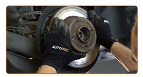
Install the brake disc assembled with the wheel hub bearing.
