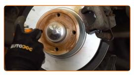
Clean the brake disk surface. Use a wire brush. Use a brake cleaner.
