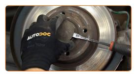
Unscrew the hub lock nut. Use a drive socket #30. Use a tap wrench.
