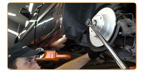
Treat the hub where it contacts the brake disk. Use a multipurpose grease.
