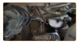
Clean the brake caliper bracket fasteners. Use WD-40 spray.
