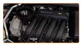
Pour oil into the engine through the filler. Required amount of oil: 4.8 L.
