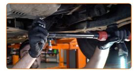
Install the lower sound insulation. Screw in the fasteners of the lower sound insulation. Use a drive socket #12. Use a ratchet wrench.
