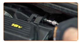
Remove the air filter housing.
