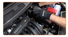
6 Disconnect the crankcase ventilation hose from the intake manifold.
