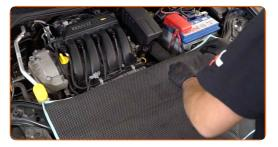
Unscrew the air filter box fasteners. Use a drive socket #10.
