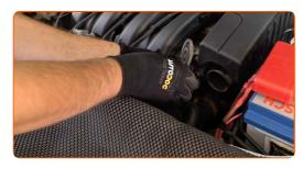
Connect the air intake pipe to the air filter box.
