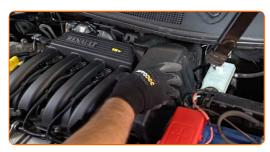
Screw in the air filter box fasteners. Use a drive socket #10.
