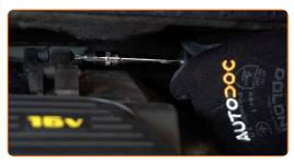
Connect the crankcase ventilation hose to the intake manifold.
