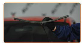
Remove the blade from the wiper arm.
