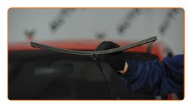
Remove the blade from the wiper arm.
