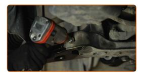
Remove the support from under the arm.
