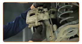
25 Install the brake caliper retaining spring. Use a flat screwdriver.
