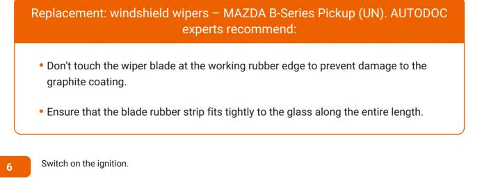
After installation check the wipers performance. The blades shouldn't intersect or bump against the windshield seal.
