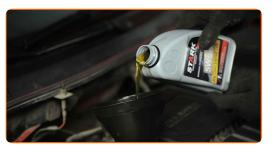
Replacement: engine oil and filter – MAZDA B-Series Pickup (UF). Tip:
