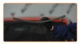
Remove the blade from the wiper arm.
