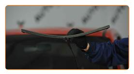
Remove the blade from the wiper arm.
