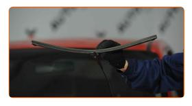
Remove the blade from the wiper arm.
