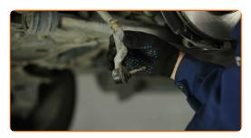
Clean the mounting seats of the tie rod end. Use a wire brush. Use WD-40 spray.
