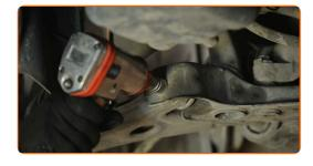
Remove the front fastener of the control arm.
