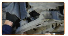
Tighten the fastener connecting the stabilizer link to the shock strut. Use a combination spanner #15. Use a drive socket #14. Use a torque wrench. Tighten it to 50 Nm torque.
