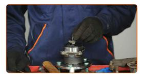
Screw in the ABS sensor fastener. Use a drive socket #6. Use a torque wrench. Tighten it to 5 nm torque.
