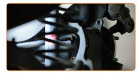
Use Torx T50. Use a torque wrench. Tighten it to 62 nm torque.
