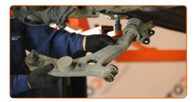
Unscrew the fasteners and remove the bump stop from the front independent suspension lower control arm. Use a drive socket #12. Use a ratchet wrench.
