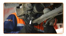
11 Remove the fastening bolt.
