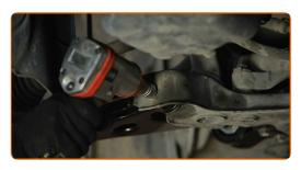
Remove the support from under the arm.
