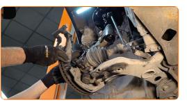
Remove the brake disc.
