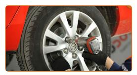
Lower the car and working in a cross order, tighten the wheel bolts. Use wheel impact socket #19. Use a torque wrench. Tighten it to 118 nm torque.
