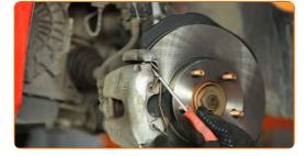
Remove the dust boot caps of the brake caliper guide pins. Use a flat screwdriver.
