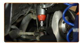
Tighten the tie rod end locknut. Use a combination spanner #24. Use a torque wrench. Tighten it to 80 nm torque.
