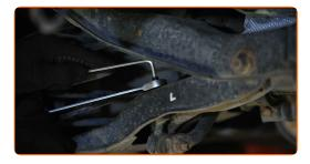
Remove the fastening bolt.
