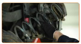
Remove the rubber spring spacer.
