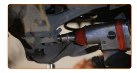
Remove the support from under the arm.
