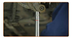
Install the fastening bolt. Use a crowbar.
