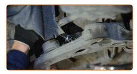
Tighten the fastener connecting the stabilizer link to the shock strut. Use a combination spanner #15. Use a drive socket #14. Use a torque wrench. Tighten it to 50 Nm torque.
