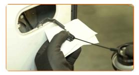
Install the bulb in the new third brake light.
