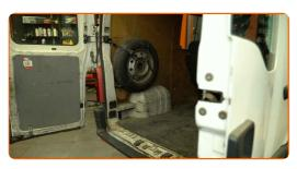
Remove the left rear door trim panel. Use a ratchet screwdriver.
