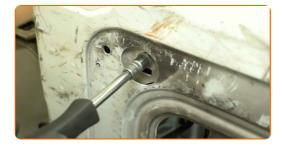
Reinstall the rear door trim cover. Use a ratchet screwdriver.
