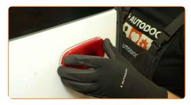
Screw on the fastener of the third brake light. Use an 8 mm socket. Use a ratchet screwdriver.
