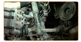
Install the spring compressor on the spring.
