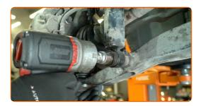
Unscrew the upper fastener of the shock absorber. Use an 18 mm socket. Use a ratchet wrench.
