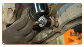
To tighten the fasteners correctly, you have to jack up the suspension to load it. Use a transmission jack or one more vehicle jack.
