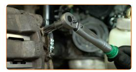
Reattach the brake bleeder screw cap.
