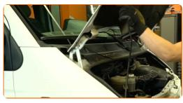
2 Loosen the brake fluid reservoir cap.
