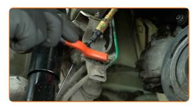
Disconnect the brake pipes from the brake hoses. Use an 11 mm flare nut wrench.
