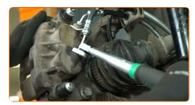
Insert one hose into the brake pipe bracket and remove the fluid line stopper on the corresponding pipe.
