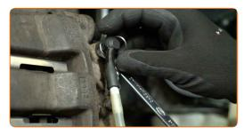
Tighten the brake bleeder screw. Use an 11 mm socket. Use a torque wrench. Tightening torque: 9 N·m.
