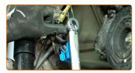
Remove the caps of the brake bleeder screws. Use a mounting lever.
