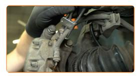
Unscrew the nut fitting that connects the brake hose to the brake caliper. Use a 10 mm flare nut wrench.
