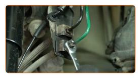
Block off the brake pipes. Use fluid line stoppers.
