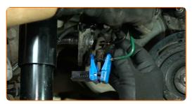
Screw in the nut fitting that connects the hose to the brake pipe. Use an 11 mm flare nut wrench.
