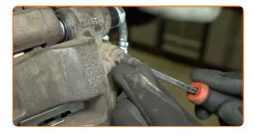
Clean the brake bleeder screws. Use a wire brush. Use an all-purpose cleaning spray.
