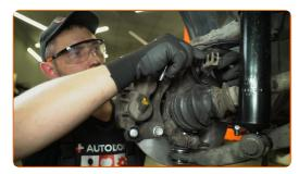
Remove the plug from the corresponding hole in the brake caliper.
