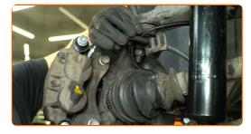
Screw in the nut fitting connecting the brake hose to the brake caliper. Use a 10 mm flare nut wrench.
