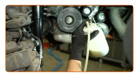
Loosen the brake bleeder screw. Use an 11 mm combination spanner.
