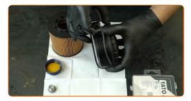
17 Install a new filter element into the oil filter cap.
