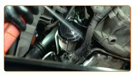
Unscrew the filter cap together with the old filter element. Use a 96-18F oil filter cup wrench. Use a ratchet wrench.
