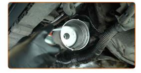
Install the oil filter cap and screw it in. Use a 96-18F oil filter cup wrench. Use a torque wrench. Tightening torque: 25 N·m.
