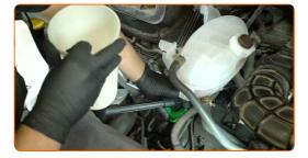
Pour oil into the engine through the filler. Required amount of oil: 8 L.
