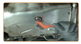
Unscrew the drain plug. Use an 8 mm square head drain plug socket. Use a ratchet wrench.
