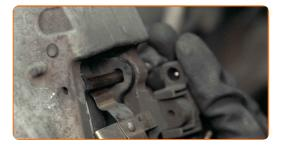
Install the wear sensor on the brake pads.
