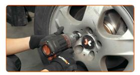
Lower the car and working in a cross order, tighten the wheel bolts. Use wheel impact socket #17. Use a torque wrench. Tighten it to 150 Nm torque.
