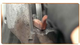
Replacement: brake pad wear sensor – Mercedes ML W163. Tip from AUTODOC experts:
