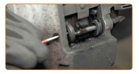
Remove the brake pads. Use a crowbar.
