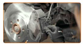
Install the brake pads retaining clips. Use a pin punch. Use a rubber mallet.
