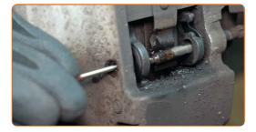
Remove the brake pads. Use a crowbar.
