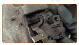
Attach the connector of the brake pad wear sensor.
