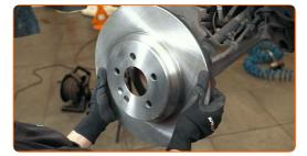
Tighten the brake disc fastening. Use HEX No.H5. Use a torque wrench. Tighten it to 8 Nm torque.
