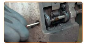
10 Remove the brake pads. Use a crowbar.
