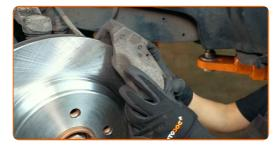
Tighten the brake caliper bracket. Use a drive socket #22. Use a torque wrench. Tighten it to 115 Nm torque.
