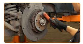
19 Install the brake disc.
