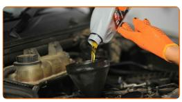
Replacement: engine oil and filter – Mercedes ML W163. Tip from AUTODOC:
