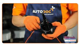
Install new O-rings (3 pieces) and a new oil filter to their mounting seats on the filter cover.
