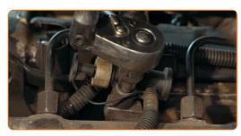
Detach the glow plug wiring connectors. Use needle nose pliers.
