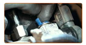
Unscrew the engine vacuum pipe fastener. Use a drive socket #E11. Use a ratchet wrench.
