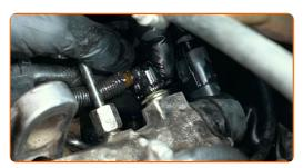
Tighten the engine vacuum pipe fastener. Use a drive socket #E11. Use a ratchet wrench.
