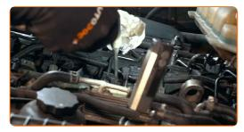
Unscrew the glow plugs. Use the spark plug socket #10. Use a torque wrench.
