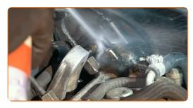
Disconnect the fuel return line hose. Use a flat screwdriver.
