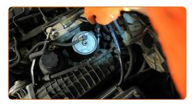
Connect the fuel supply lines to the fuel filter and tighten the fasteners. Use a flat screwdriver.
