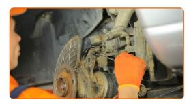
Install the ABS sensor on the steering knuckle and secure it. Use a drive socket #10. Use a drive socket #E10. Use a ratchet wrench.
