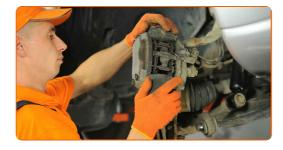
Tighten the brake caliper bracket. Use a drive socket #21. Use a torque wrench. Tighten it to 180 nm torque.
