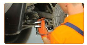
Unscrew the ABS sensor fastening from the steering knuckle. Use a drive socket #10. Use a drive socket #E10. Use a ratchet wrench.
