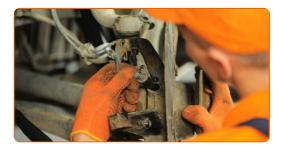
Tighten the hub. Use a drive socket #36. Use a torque wrench. Observe the recommended tightening torque.
