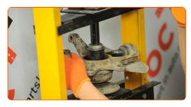
Install the steering knuckle with a hub in assembly.
