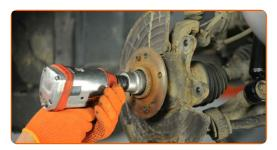
Unscrew the end fastening nut to the steering knuckle. Use a drive socket #22. Use a ratchet wrench.
