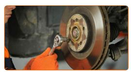
Remove the brake disc. Use a hammer.
