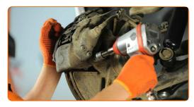
Remove the brake caliper together with its bracket. Use a flat screwdriver.
