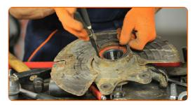
Press the wheel hub into the bearing inner race. Use a bush and bearing driver set.
