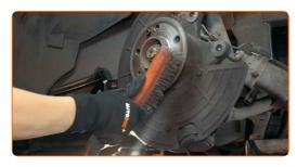
18 Install the brake disc.
