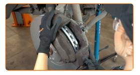
Tighten the brake caliper bracket. Use a drive socket #22. Use a torque wrench. Tighten it to 180 Nm torque.
