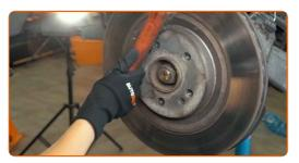
Unscrew the brake disc fastening. Use HEX No.H5. Use an impact screwdriver.
