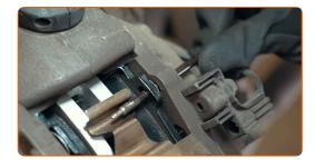
Attach the connector of the brake pad wear sensor.
