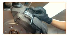
Install the brake pads retaining clips. Use a rubber mallet.
