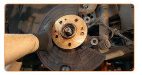
Screw in the fasteners of the brake disc cover. Use a drive socket #12. Use a torque wrench. Tighten it to 9 Nm torque.
