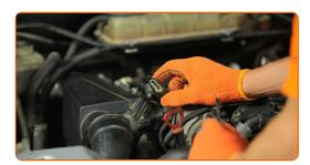
Undo the fastening screws of the air filter cover. Use a drive socket #E11. Use a ratchet wrench.
