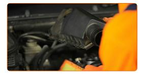
Remove the filter element from the filter housing. Use a flat screwdriver.
