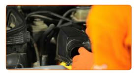
Screw in the fastening screws of the air filter cover. Use a drive socket #E11. Use a ratchet wrench.
