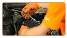
Plug in the mass air flow sensor conntector.
