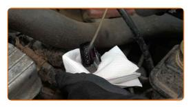
Plug in the ignition coil connector.
