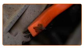
Unscrew the ignition coil bolts. Use a drive socket #10. Use a ratchet wrench.
