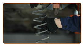
Remove the rubber spring spacer.
