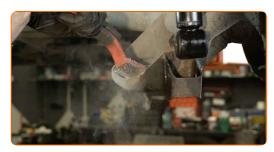
15 Install the rubber spring spacer.
