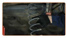
Clean the coil spring mounting seats. Use a wire brush. Use WD-40 spray.
